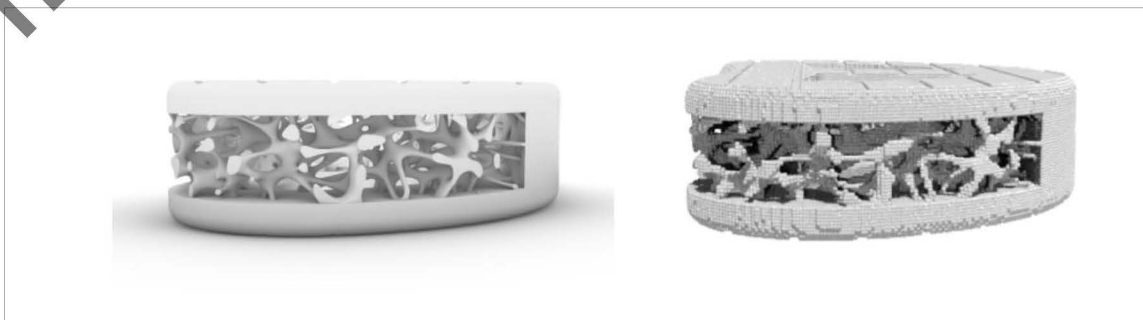
Figure 3. Example STL to 182 μm particle model conversion for a representative 3D-printed spinal spacer device
